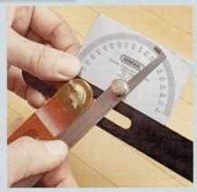
A protractor is best for intermediate angles, just rest the blade against the base and lock in the setting.
