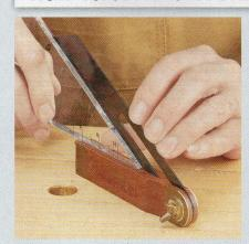
A drafting triangle is an easy and accurate way to set a specific angle, such as the 30° angle shown here.
