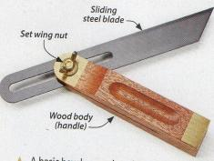
A basic bevel gauge is a simple tool consisting of a body and blade with a locking mechanism. **THE SOLUTION.** In most cases, you'll find that a bevel gauge is the tool of choice to solve the problem (photo at left). A bevel gauge is also referred to as a sliding T-bevel, carpenter's bevel or sliding bevel gauge. Regardless of the name, its purpose is to duplicate an angle exactly, without having to do any measurement.
