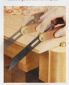
Sliding a bevel gauge along a hand-planed bevel makes quick work of checking the accuracy of your work.
