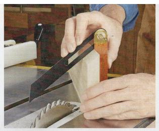
Don't know the existing bevel angle of a workpiece? No problem. Loosen the bevel gauge and rest the blade and body against the desired angle and then lock it in place.
